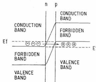
**FIGURE 6.** Tunneling current in a reverse-bias, backward tunnel diode used as a rectifying device at zero bias (Morizuka, K., "Rectifying device for achieving high power efficiency," U.S. Patent 5,930,133, July 27, 1999, Figure 5)
