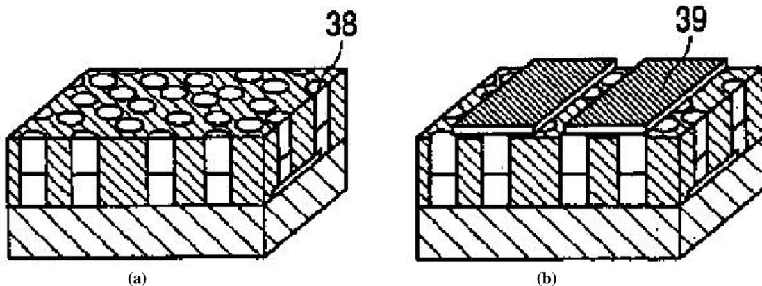
**FIGURE 4.** Updated version of a Brown's p-n junction (a) diode array (38) and (b) with parallel conductors (39) added (Kuriyama, A., Miyata, H., Otto, A., Ogawa, M., Okura, H., Fukutani, K., and Den, T., "Method for Manufacturing a Semiconductor Device", U.S. Patent 7,183,127, Feb. 27, 2007, Fig. 4D and 4E).
