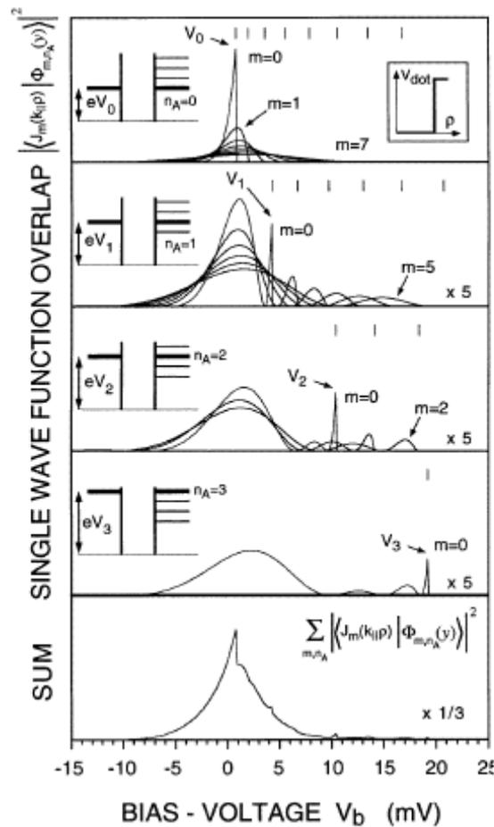
**FIGURE 7.** Calculated wave function overlap between the 2D state and the lowest three 0D states for a quantum dot with a rectangular potential of finite height (for example, an ultra-small, pillar-shaped double-barrier resonant tunneling diode), including the sum over all 0D subbands showing a maximum at zero bias voltage (Smoliner, 1996).
