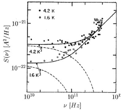
**FIGURE 2.** Measured spectral density of current noise in the shunt resistor of Josephson junction at 4.2K (solid circles) and 1.6K (open circles) up to 500 GHz. Solid lines are the prediction of Equation 2 while the dashed lines represent the theoretical prediction in the absence of the zero-point energy term and fall far below the data at the higher frequencies (Koch, 1982).
