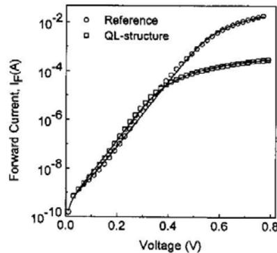
**FIGURE 9.** Experimental forward current-voltage characteristic of a typical Au/n-GaAs Schottky diode for a reference GaAs sample and the GaAs with InAs QL structure sample showing  $10^{-10}$ A current conduction at zero bias voltage (Hastas, 2003).
