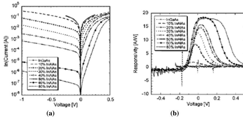
**FIGURE 5.** Example of a modified Schottky diode (semimetal-semiconductor) InGaAs rectifier for sensitive room-temperature microwave detection that operates well at zero bias voltage, where (a) shows increasing current levels in amperes with lower InAlAs percentage and (b) shows increased responsivity in A/W at zero bias voltage and higher InAlAs levels (Young, 2005).
