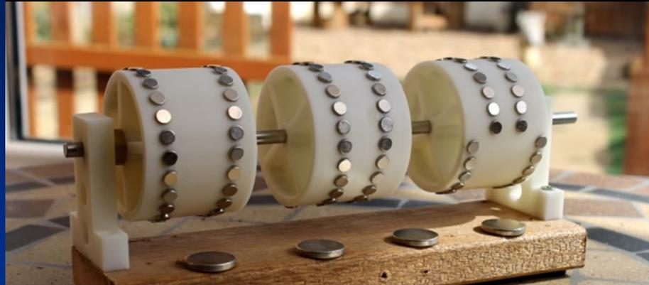
The trigger magnet / magnets face the opposite direction to that of the drum magnets - repelling force
