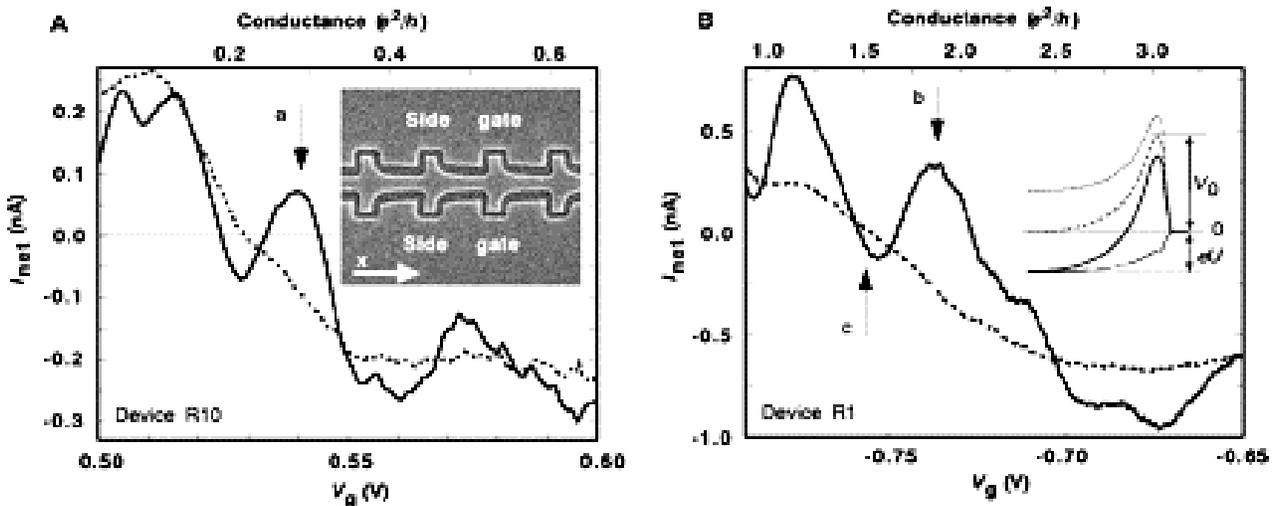
Figure 45 Net current for quantum ratchet. Solid lines,  $T = 0.4\text{K}$ . Dotted lines,  $T = 4\text{K}$ . Inset SEM shows four repeating ratchet cells. Temperature-dependent current reversal at a, b, c.
