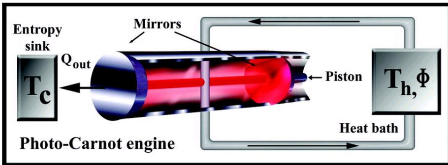
Figure 42 Photo-Carnot heat cycle diagram. Q<sub>in</sub> is provided by hot atoms
