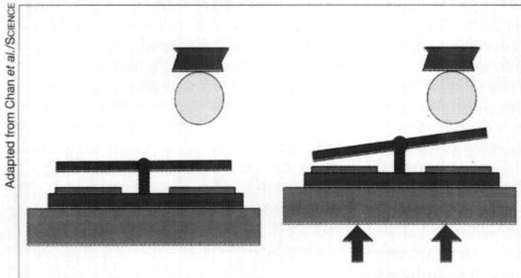
*A chip with a see-saw plate suspended parallel to its surface (left) is pushed up (right) toward a ball. Quantum fluctuations in empty space produce a force that tilts the plate.*
