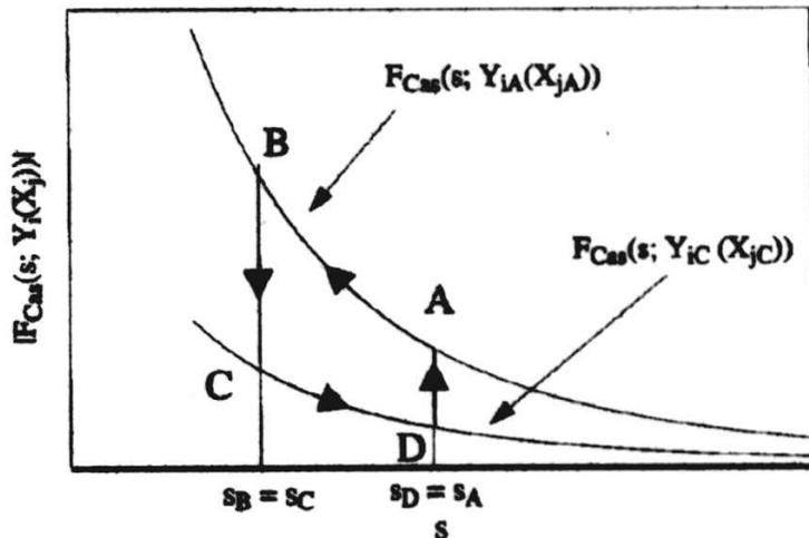
Figure 31 – Thermodynamic engine cycle of Pinto's vacuum energy transducer where  $F_{Cas}$  = Casimir force
