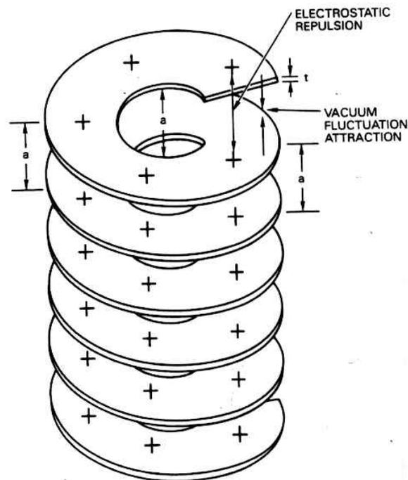
Figure 8 Spiral design for a vacuum-fluctuation battery.
