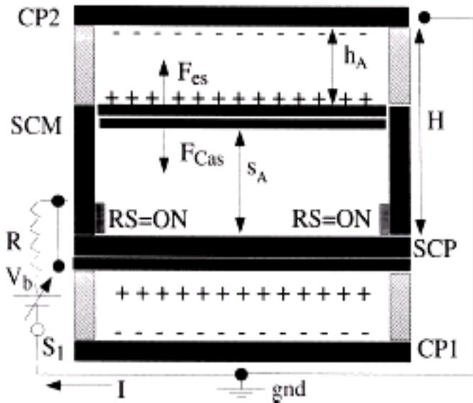
Figure 30 – Pinto's optically controlled vacuum engine
