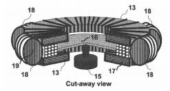
discloses an apparatus and method for electromagnetic spacecraft propulsion. The apparatus includes capacitor assemblies bracketed by electromagnetic solenoids configured in Helmholtz Coil geometries. The action of magnetic fields generated in the solenoids on segmented currents in conductive discharge elements during capacitor discharge produces unidirectional forces, while reaction momentum is
