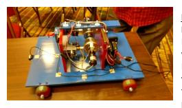
Propulsion Program. The Control Moment Gyro **Project** successfully produced a tabletop prototype by Mike Gamble (see left), the retired Boeing Engineer who is the Chief Engineer on the project. For years, Inertial Propulsion has been advocated by IRI and now we have replicated a table-top model. The purpose of this experiment is to show that forward thrust and propulsion is possible by scissoring gyros, as Boeing
