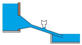
Cross section of the Venturi tube. When the water flows through the uptake tube, negative pressure builds that forces the elastomer film (center of the image) to extend inwards. Credit: Fraunhofer ISC
