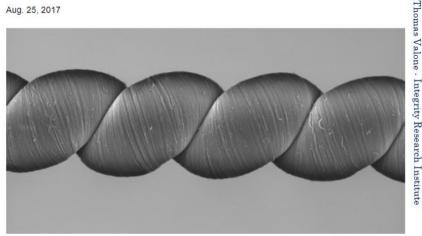
Coiled carbon nanotube yarns, created at The University of Texas at Dallas and imaged here with a scanning electron microscope, generate electrical energy when stretched or twisted.
