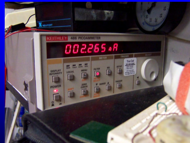
Keithley 486 Picoammeter reads 2.27 nanoamps constant current with or w/o resistor in series
