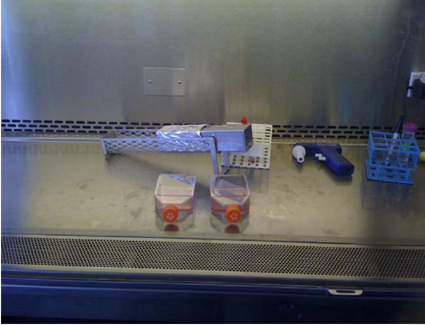
Negative control cell cultures under an adjacent hood during exposure time of experimental cultures
